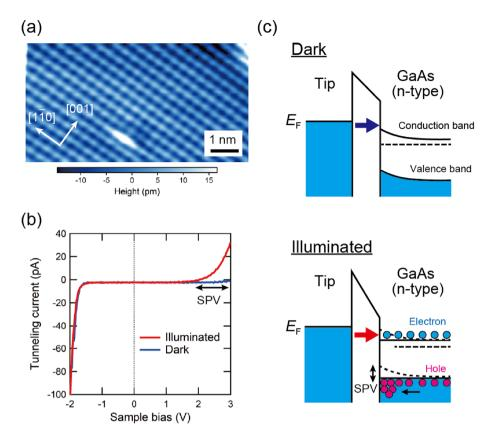
**Figure 5.** (a) Constant-current STM image of GaAs(110) surface. Set-point: sample bias voltage V = -3 V, and tunneling current  $I_t = 100$  pA. T = 78 K. (b) I-V curves obtained with (red) and without laser illumination (blue). Set-point: V = -2 V,  $I_t = 100$  pA. T = 78 K. (c) Schematic illustrations of the band structures of the n-type GaAs surface when V > 0 without (top) and with laser illumination (bottom).
