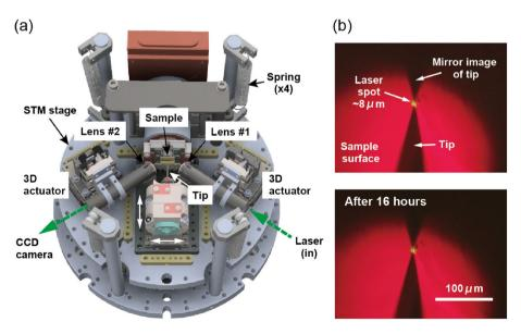
**Figure 3.** (a) Three-dimensional illustration of the STM unit (top-view). Electrical wirings and copper heat links are not shown for clarity. (b) (Top) Optical image of the tip and its mirror image on GaAs(110) surface with a laser spot illuminated at the tunneling junction. (Bottom) The image taken after 16 hours, showing the stability of the laser spot.
