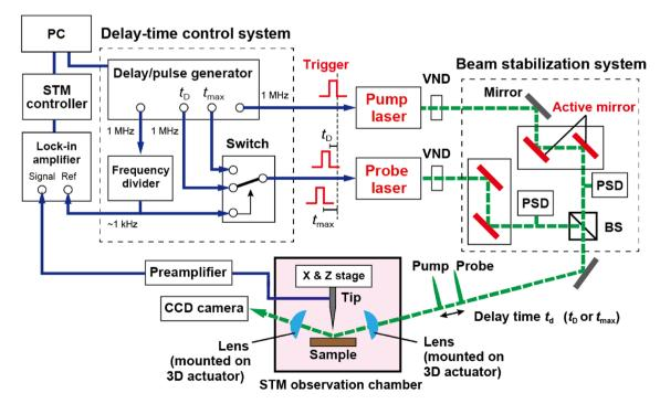
**Figure 1.** Schematic diagram of the OPP-STM system. PSD: position sensitive detector, BS: beam splitter, VND: variable neutral density filter.
